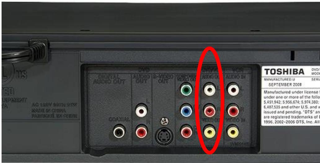
b. Toshiba's audio/video connectors are at the back of the VCR.
